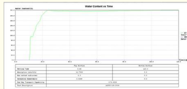
Figure 7: Water content vs time graph of nanofiber with a mask.
