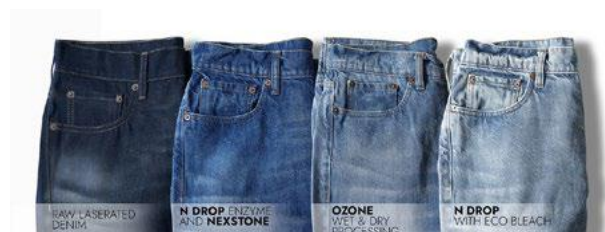
Figure 3: NEXSTONE, Stone free abrasion, an exclusive and unique patented system whereby textiles are washed without the use of pumice stone, Nexstone also allows for the reduction of waste emissions as well as limiting water consumption.
