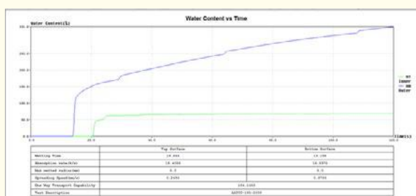
Figure 5: water content vs time graph of the only nanofiber.
