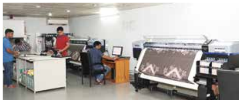
Figure 3: Dye-sublimation printer can produce 70000 pieces of garment per month.
