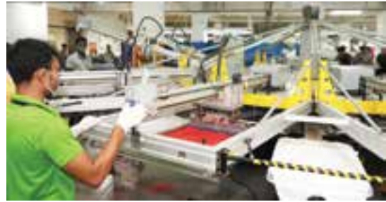
Figure 4: Operator is checking the print process in the Octopus machine.
