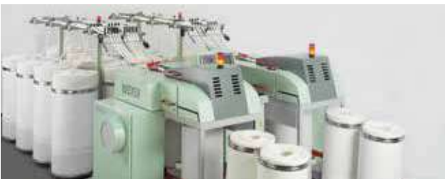
Figure 2: RSB-D 22 operating at a higher speed after the implementation of draw frame mini kit.
