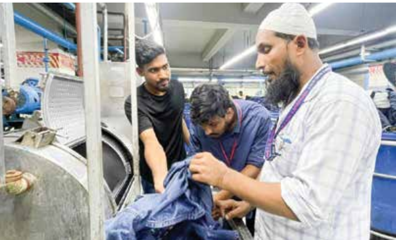
Figure: The enzyme wash method significantly reduces water usage by saving one water batch and two rinse cycles,
